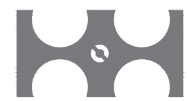
Purpose made 4 way spacer to be used a 3m intervals
