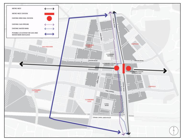
Figure 3.10: Illustration showing the preferred alignment of Metro West and the location of the station, the existing alignments of the gas and water mains and the possible re-routing of them to the west of the UFDF area.
