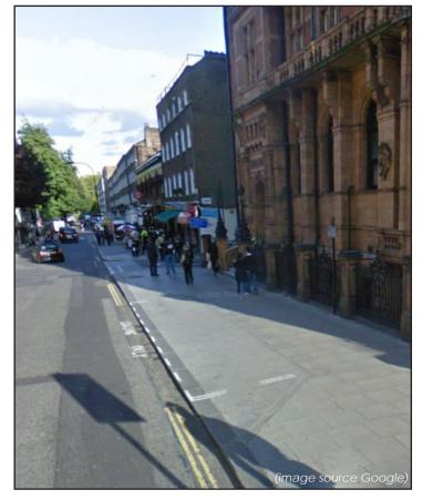
Figure 4.15: Example of an on-street loading bay that when not in use reverts to part of the footpath.
