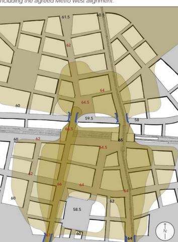
Figure 4.4: Application of approximate levels to the block structure where a constant height is maintained between bridges spanning the canal and railway.
