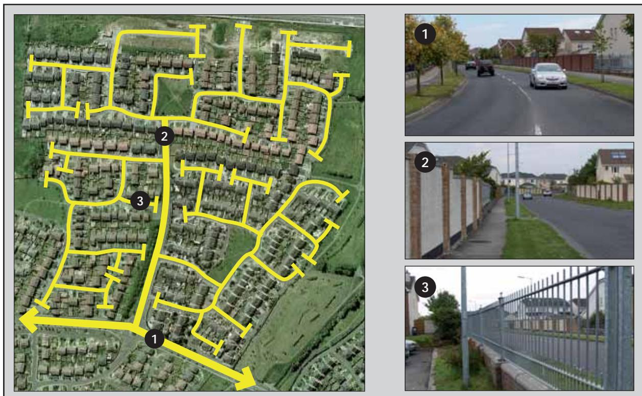
Figure 2.4: Example of a residential community designed according to the keynote principles of segregated street networks. 1) Distributor roads are designed to facilitate free flowing traffic and provide access to 2) neighbourhood cells. Movement through the cell enforced via a dendritic street layout of 3) cul-de-sacs that spread out like the branches of a tree (base image source: Google Maps).
