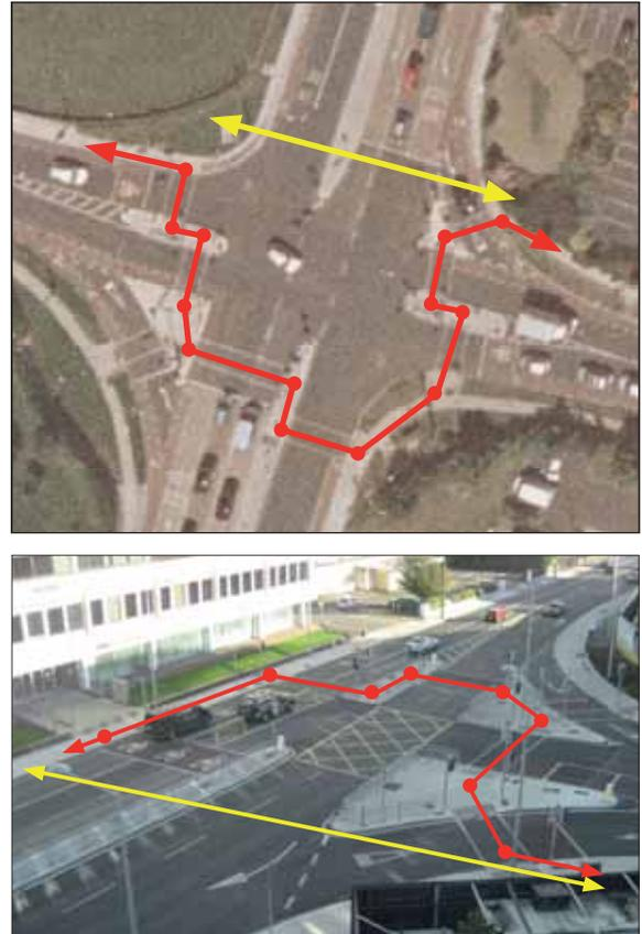
Figure 2.8: Examples of a junctions designed to minimise vehicle delays which significantly increase crossing times for pedestrians. Pedestrian desire lines (represented by the yellow line) are diverted through a series of separate crossings (represented by the red line). The top example can take pedestrians as long as 5 minutes to navigate.
