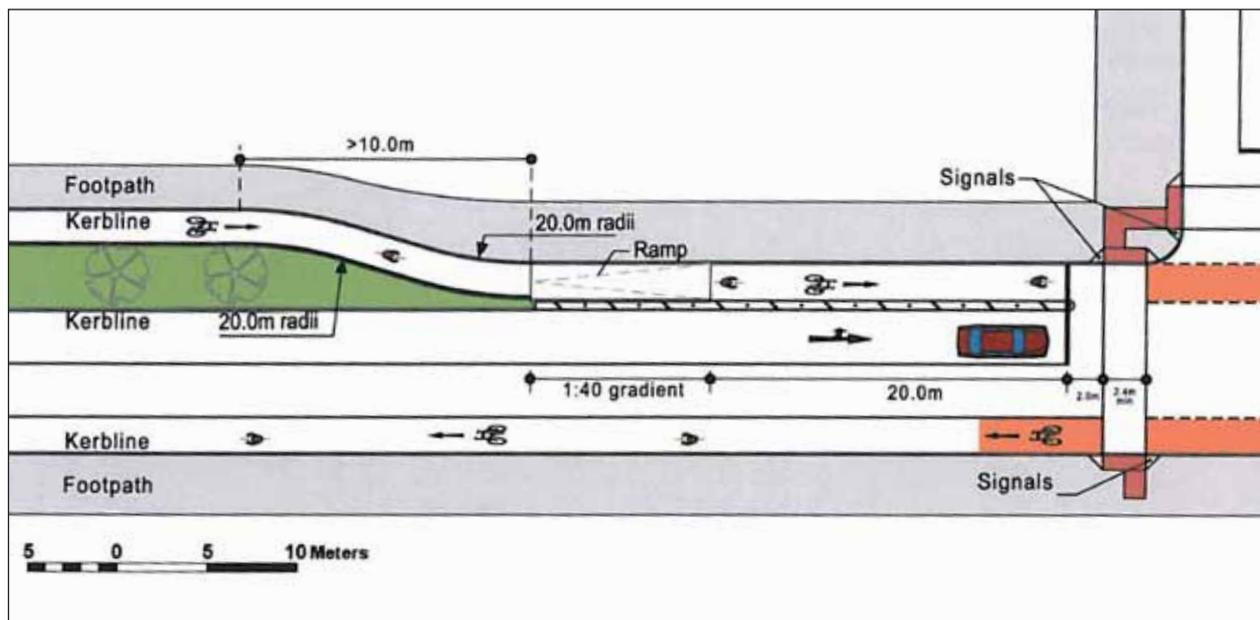
Figure 4.54: Extract from page 86 of the *National Cycle Manual* illustrating how to re-establish from an Off Road Cycle Track to Cycle Lane on approach to a junction. This design can be adapted to cater for on-street parking by placing spaces within the green area or verge between the vehicular carriageway and Cycle Track.
