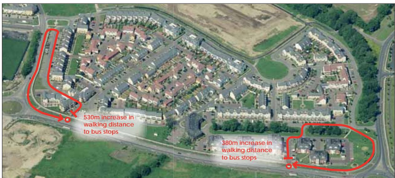
Figure 2.7: Example of a 'neighbourhood cell' located within a 'distributor road' network. A long fence separates the Cell from the Distributor Road. A number of openings in the fence were initially planned to provide access to bus stops. These were removed at the request of residents due to safety concerns, significantly increasing walking distances to bus stops (base image source: [www.bing.com/maps](http://www.bing.com/maps)).
