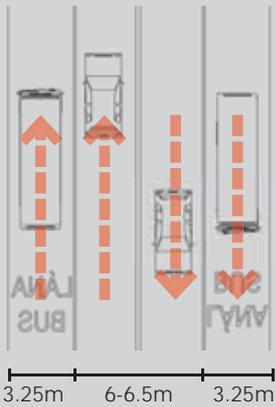
Standard lane/carrageway widths for multi lane *Arterial* and *Link* streets, including bus lanes. Range for low to moderate design speeds.
