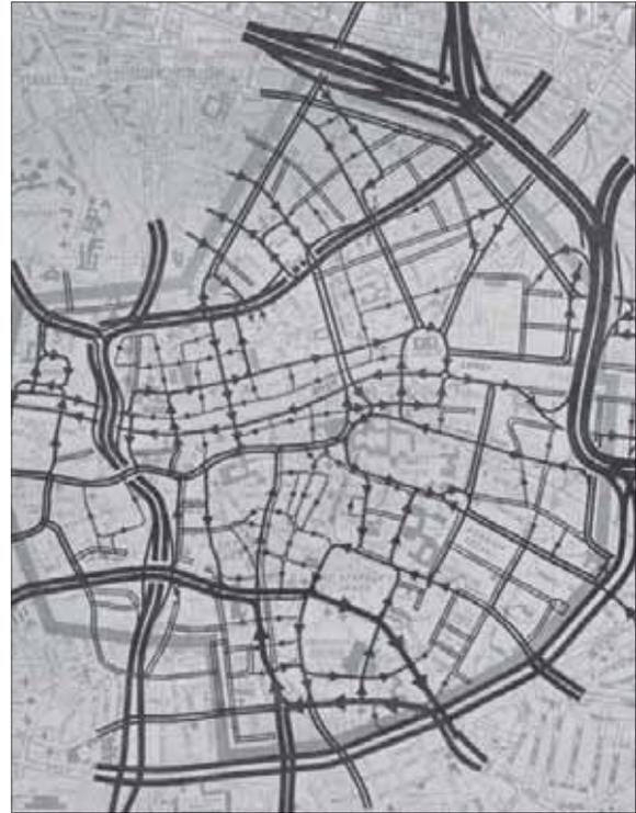
*Figure 2.3: Dublin Transport Strategy (1971). Although the scale of vision was never realised many aspects such as one-way traffic systems were implemented.*
