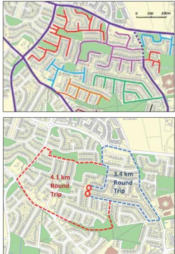
Figure 2.5: A typical example of a residential area constructed in accordance with the principles of segregation. Walking and cycling permeability is restricted to the point that the two neighbouring houses shown back to back are up to 4km walking distance apart.
