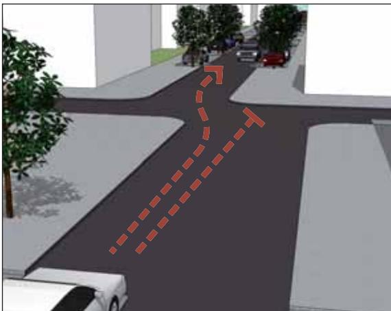
Figure 4.68: illustration of how off-setting junctions can create a change in alignment (without reducing permeability or legibility) and reduce forward visibility.
