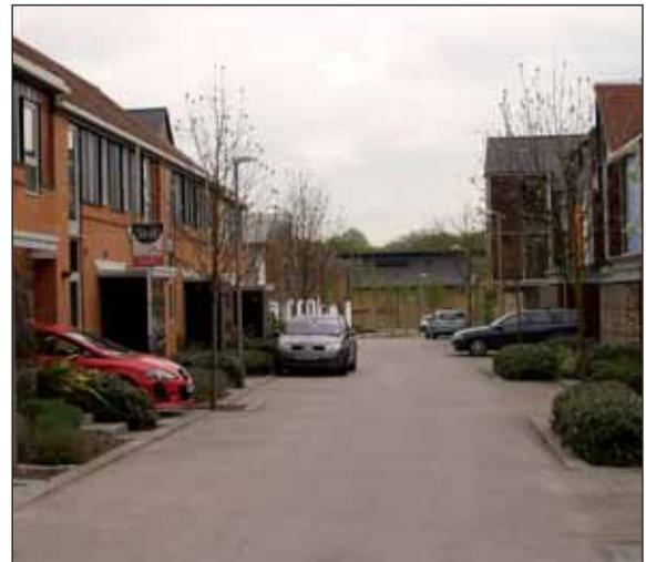
Figure 4.79. Example from New Hall, UK where a variety of in-curtilage and on-street parking is provided. On-street parking is provided semi-informally (indicated by the planting of trees). The parking of vehicles further calms traffic by providing a series of horizontal deflections.
