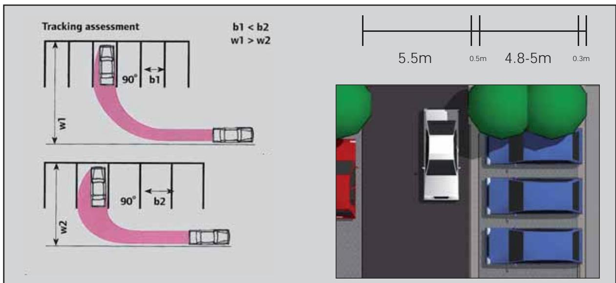
Figure 4.82: Example of how additional manoeuvrability may be provided for vehicles in areas of perpendicular parking whilst minimising carriageway widths. The images to the left are extracted from the *Manual for Streets (2007)* and illustrate the provision of wider spaces. The image to the right also shows the use of small verges.
