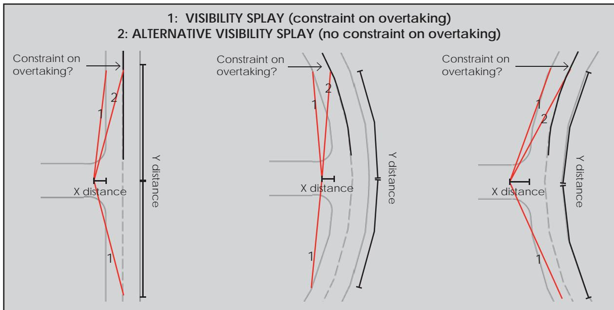
Figure 4.63: Forward visibility splays refer to an X and Y value. The X value allows drivers to observe traffic on the intersected arm. The Y value allows the driver of a vehicle to stop safely should an object enter its path, and is based on the SSD value.
