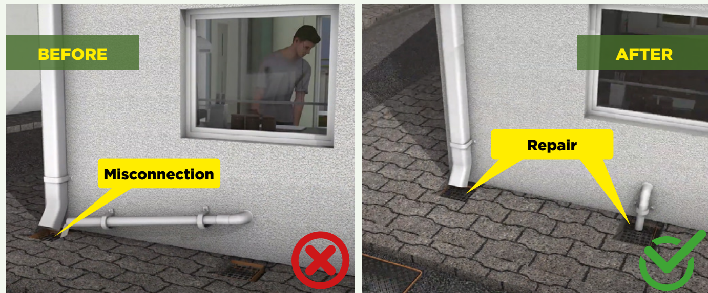
Typical domestic misconnection
