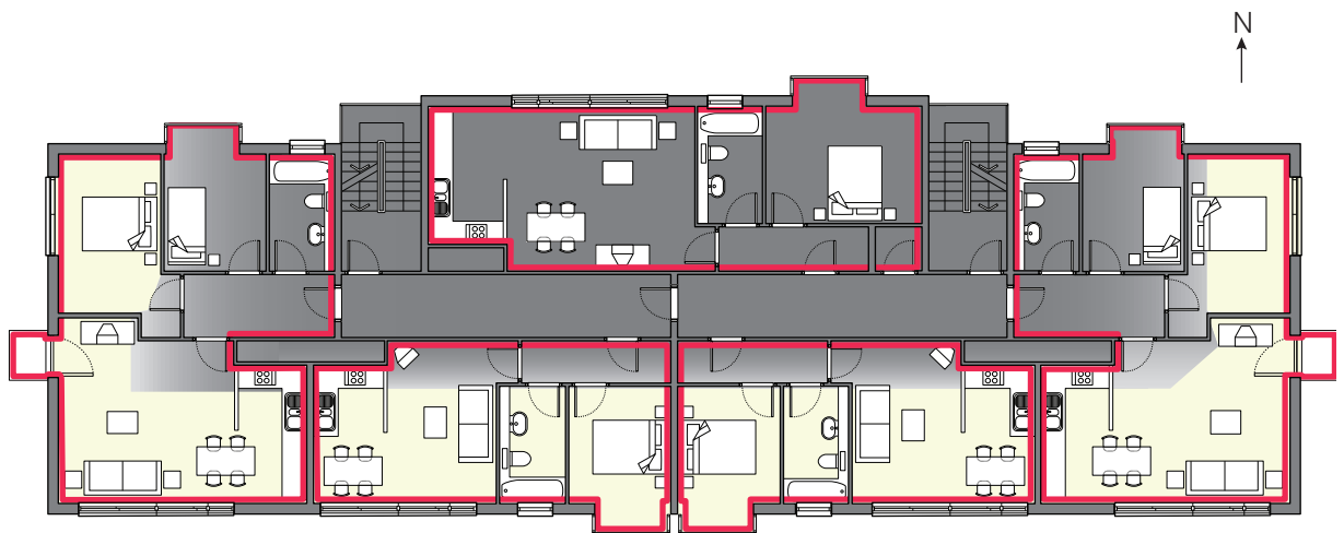
Figure 26: Careful layout design means that four out of the five flats shown have a south-facing living room
