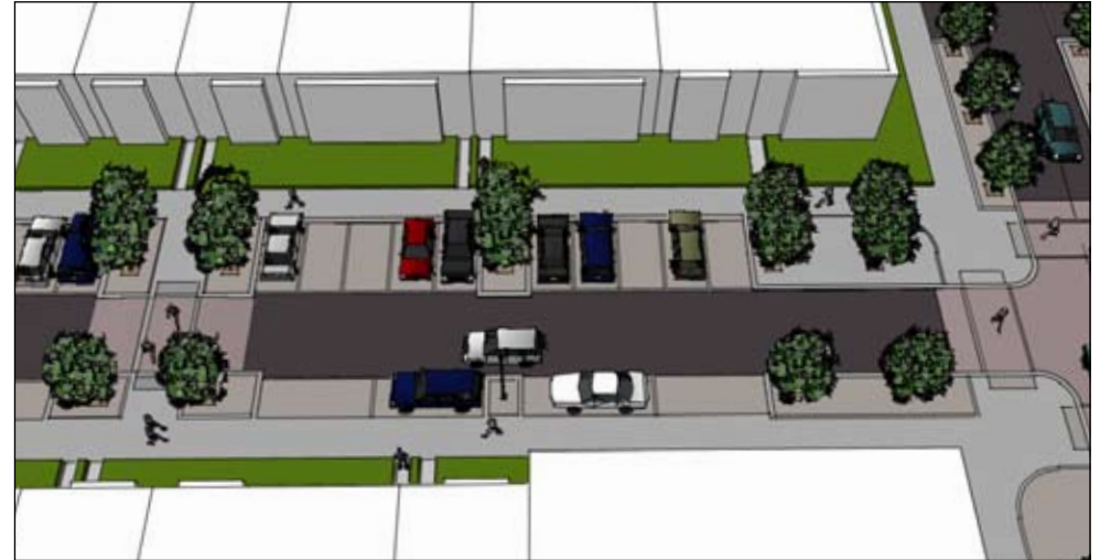
Illustration of opportunistic street tree planting along Side Street (ie at crossings, between parking bays and on approach to junctions).
