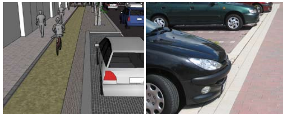
Illustration (left) and example from Adamstown (right) of a small verges between areas of on street parking and cycle lanes/pedestrian paths to allow for opening doors and vehicle overhangs, respectively.
