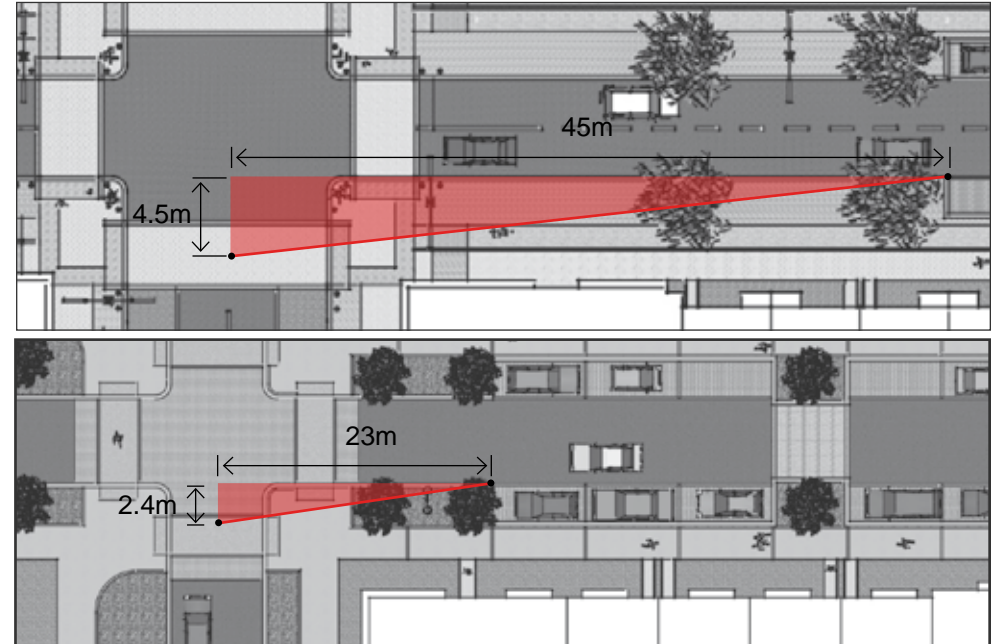
Illustrations of the main two types of visibility splays used within Adamstown for 50 kph Adamstown Boulevard/Main Streets (top) and 30 kph Side Streets/Back Streets (bottom).
