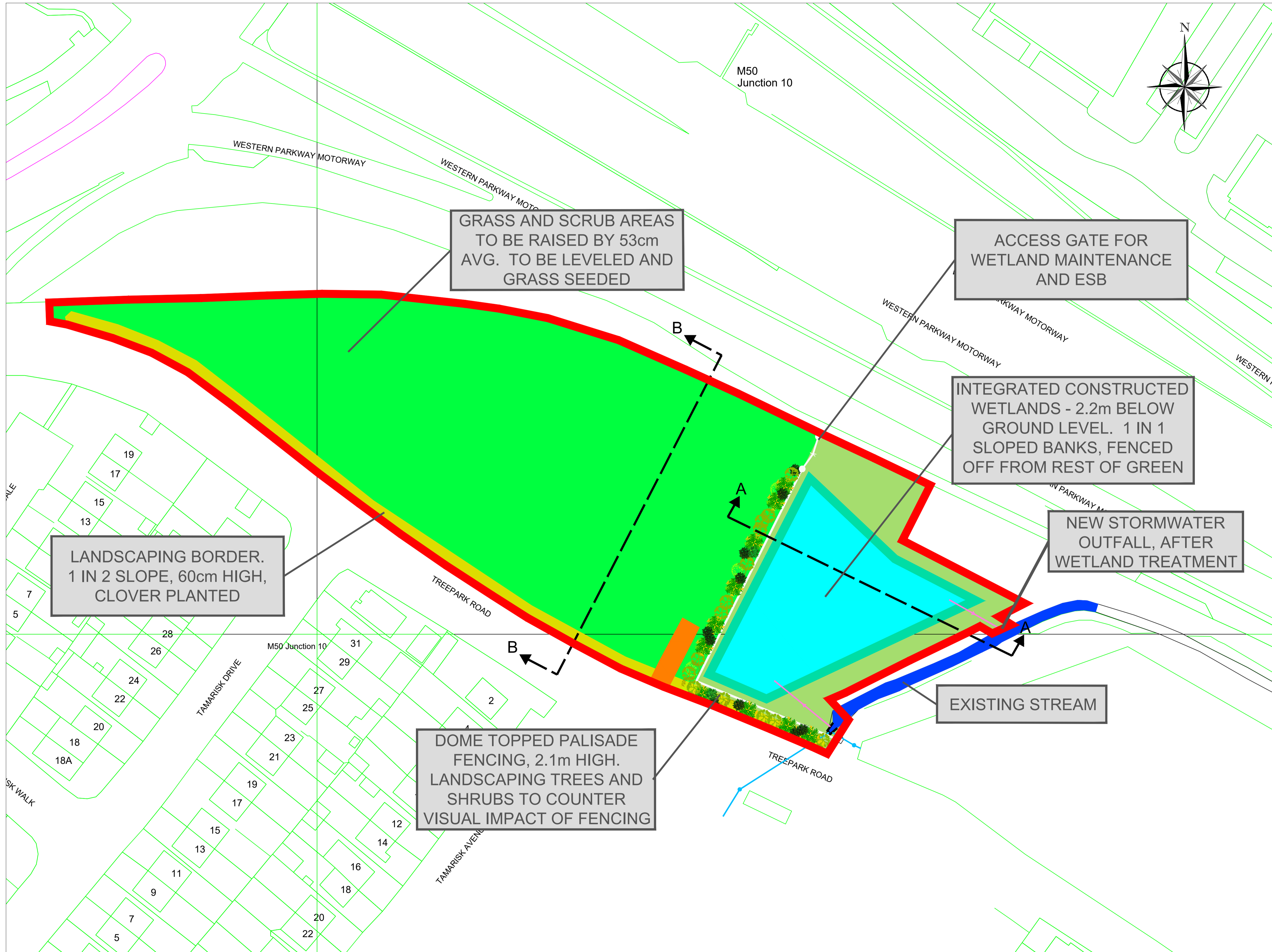
1 Proposed Site Plan - Intergrated Constructed Wetland
