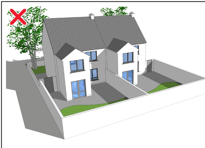
A 'tunnel effect' can be created along terraces by two-storey rear extensions
