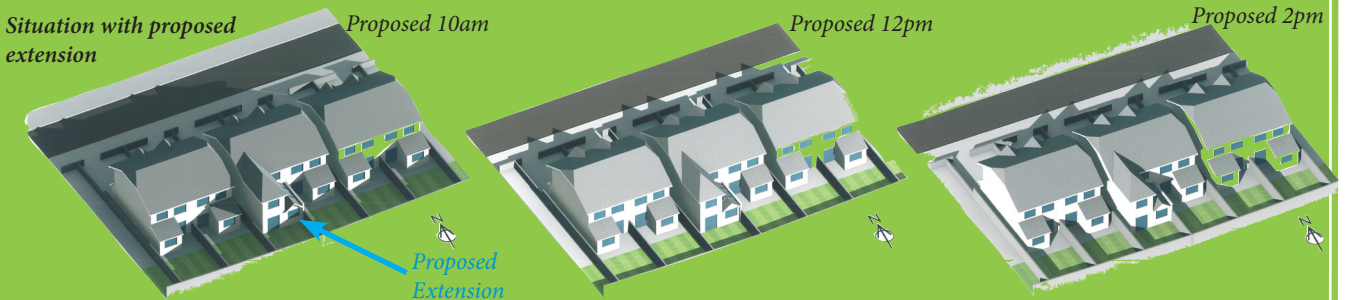
Sun shadow diagram illustrating the impact of a proposed extension at different times of the day on March 20th
