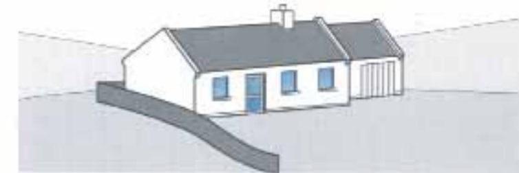
Often a garage will look better set back to read as a separate unit from the house, though still connected to it. This can lend interest and reduce bulk. It emphasises that the house is the important unit and the garage subsidiary.
